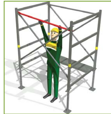
> 5 - Pose des lisses garde-corps.
